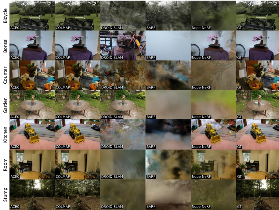
Fig. 6: View Synthesis Quality on the MIP-NeRF 360 dataset. For each scene, we show the test image where ACE0 achieves its median PSNR value. For comparison, we show the corresponding results of our baselines as well as the true test image (GT). These results correspond to Table 2 (b) of the main paper.
