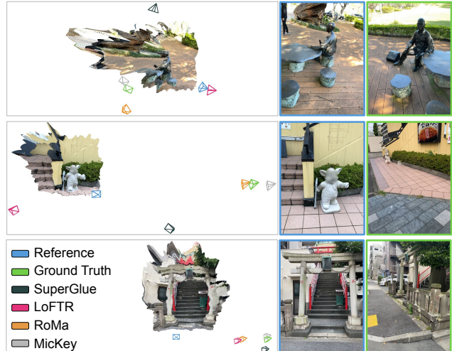
Figure 6. Visualization of relative camera poses. In this visualization, we use Map-free validation scenes and visualize the different predicted poses w.r.t. the ground truth (green camera).
