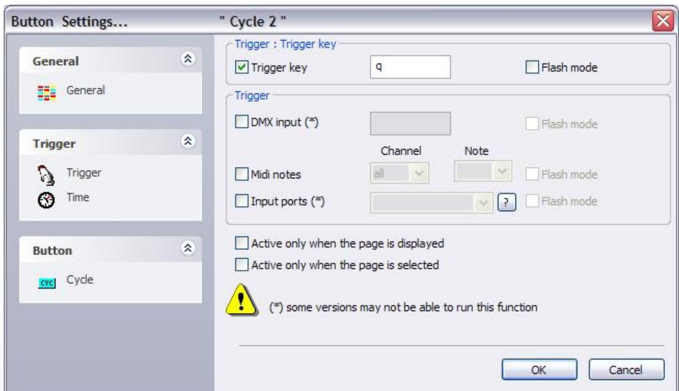
Select the "Trigger" option on the left, then tick the "Trigger key" box on the top, and assign whatever letter you want. "Flash mode" creates keys which are only active while the keys are physically being pressed; the moment you release your finger from the keyboard, they will automatically become inactive (only works with Switches, not Scenes). Try this FLASH key option with the Strobe effect, for example.
