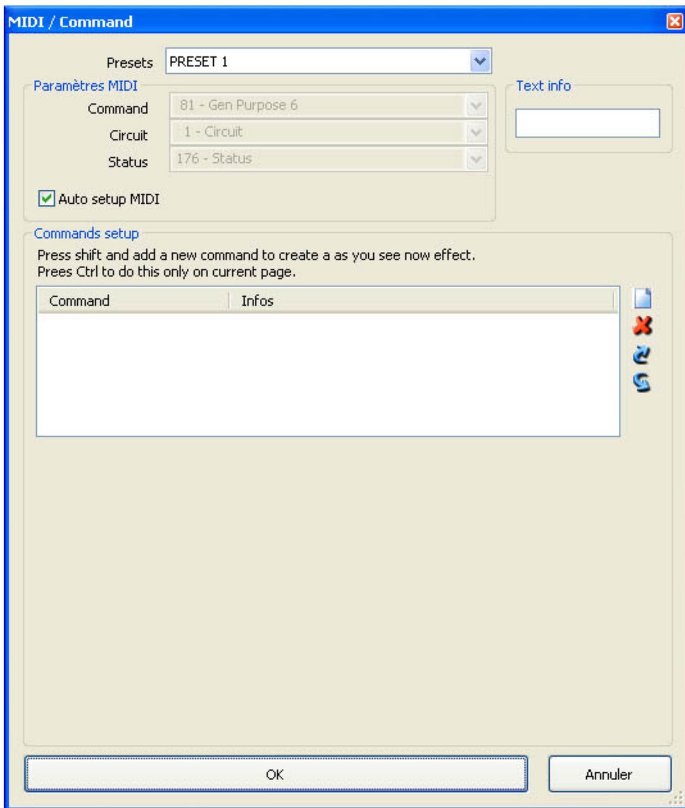
Once this window is opened and if the "Auto setup MIDI" option is activated, turn on the corresponding fader or button on your controller and it will be automatically assigned. Repeat the operation for all controls. Do not forget to save the configuration by clicking with the right button of the mouse on the title bar and selecting "Save" from the menu.
