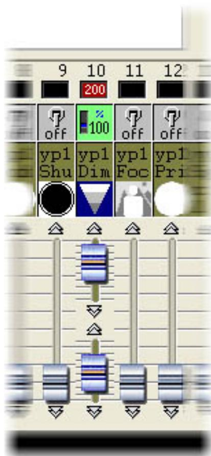
Set the minimum and maximum levels to 100 and 200 DMX, respectively, then close the Editor and save changes. You now have a button that can control a dimmer between DMX values 100 to 200. You
