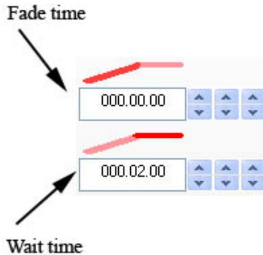
Other available functions on the EasyStep rack are copy, cut, paste and insert step. The PLAY button allows you to preview your scene. You can choose to make your scene loop or not. Finally you can convert your EasyStep scene into an EasyTime sequence (advantages of EasyTime will be explained in the Advanced Programming section).
