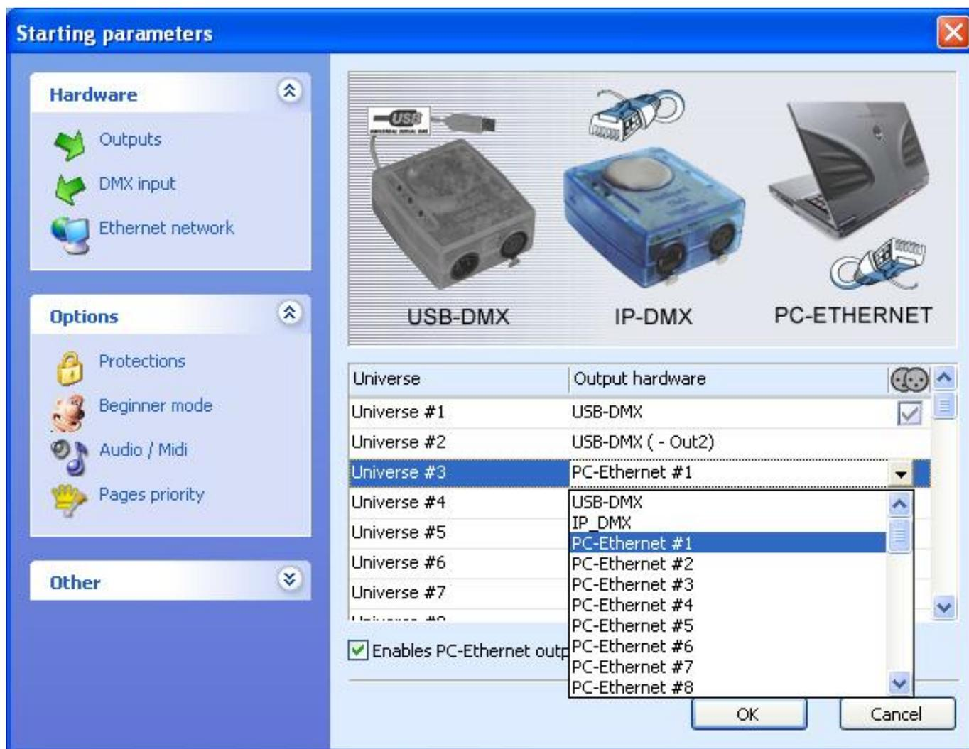
Most of the time, your fixtures won't be able to read the Art-Net protocol and you will have to convert it to DMX using an Art-Net to DMX converter. They usually convert multiple universes (2, 4, 6, 8...). We can also provide a single universe converter with our IP interface.
