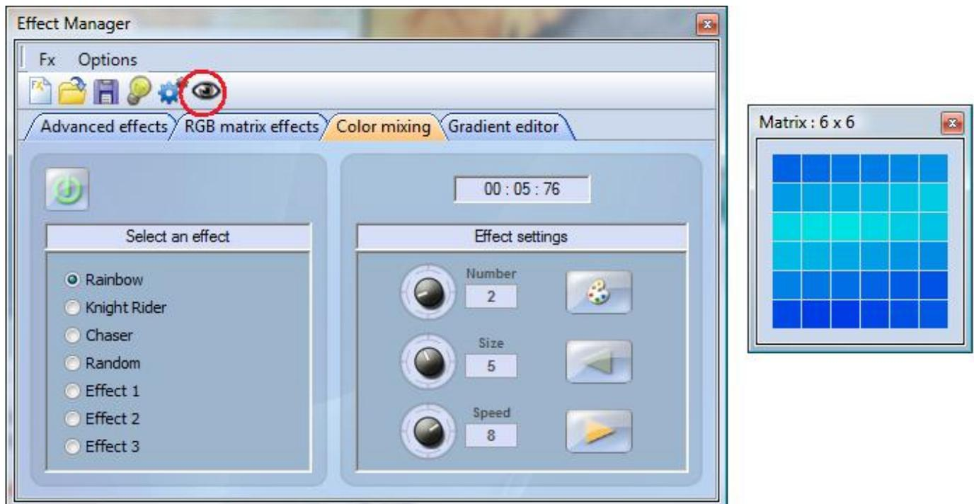
You can vary the size, speed and direction of the effect as well as changing the colours used by clicking the pallet icon. You can also change the number of colours used. Remember to click generate before closing the effect manager.
