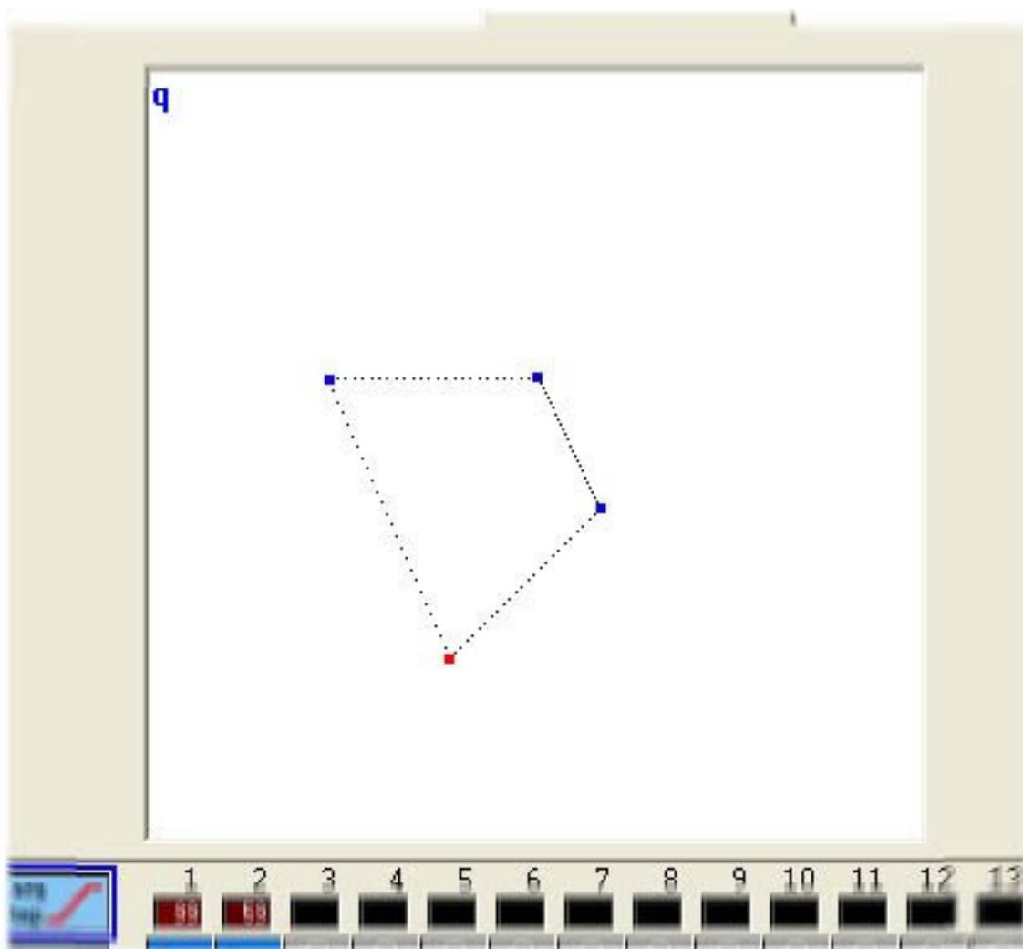
Each corner in the picture represents the X-Y position in each step. These can be moved individually with the mouse. Steps with fade in between show dotted lines in between the corners in the shape area. Steps can be selected by clicking on the corresponding point (white area) or directly from the step list at the top.
