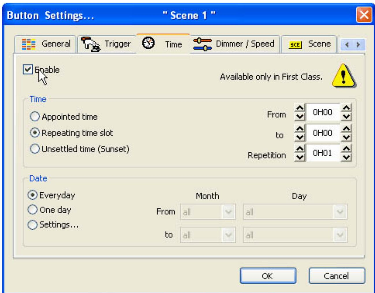
First of all, we must click on "Enable" to modify the settings. Several options are available to trigger a button (scene, switch or cycle):
