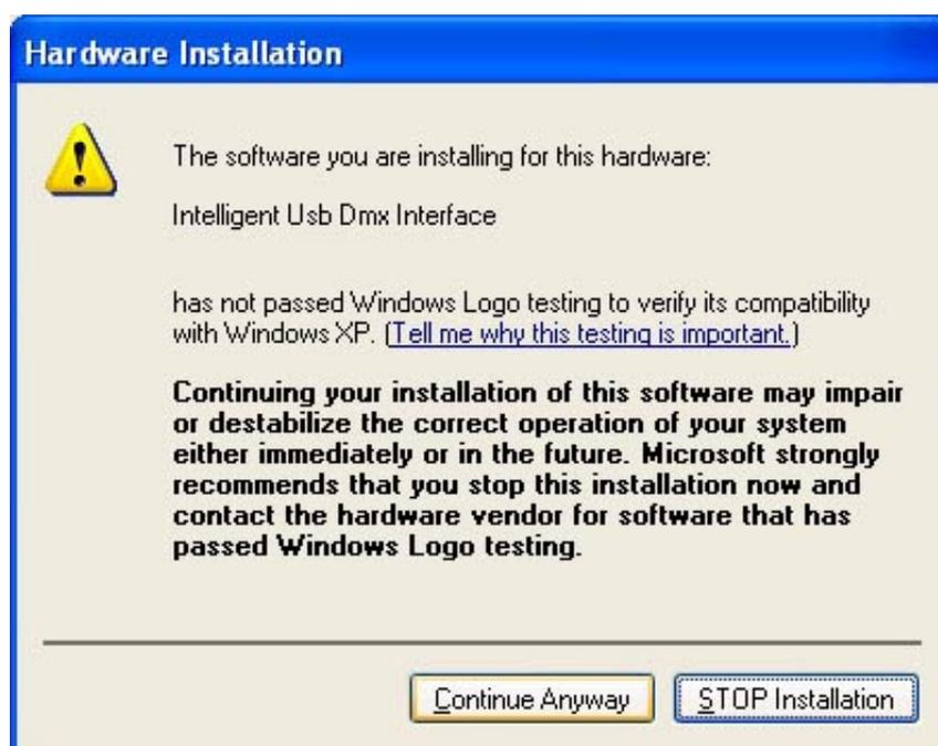
You are done! But remember, the software detects the USB interface when it starts. This means that you must have the USB interface connected to your computer before you open the control software. Otherwise, there will be no communication between the software and the interface.
