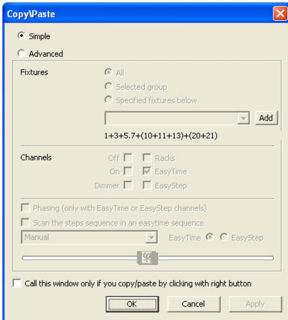
By default, "Simple" is selected. That means that the sequence will be pasted to the selected fixture. If you want to paste the same sequence to more than one fixture you have to select "Advanced" and then select the fixtures. Three options are available:
