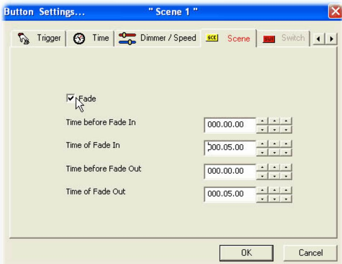
Once the "Fade" function has been selected, we can setup the fade times. Please keep in mind that the channels can have their levels increasing (Fade In) or decreasing (Fade Out):
