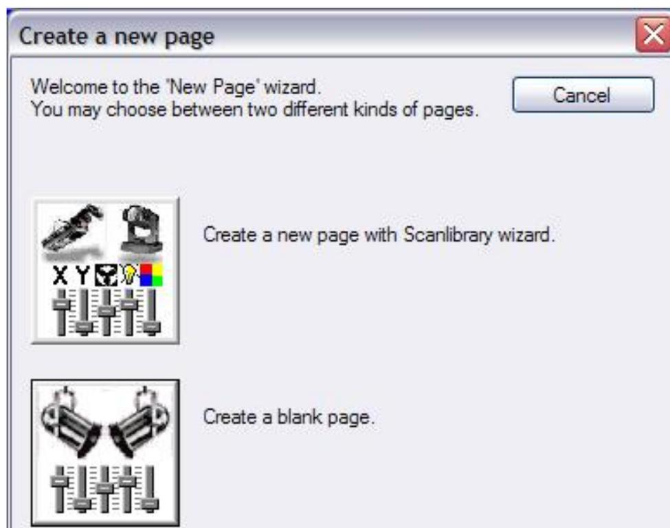
You can see two buttons. The first "Create a new page with Scanlibrary wizard" opens our profile library. The second "Create a blank page", adds an empty page of DMX channels in the software (configuration for these blank pages is described in later chapters).
