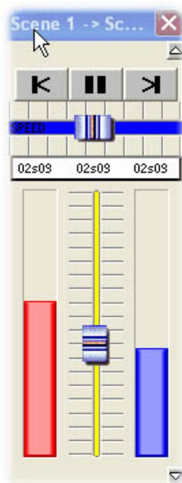
Please keep in mind that the FADE function is not available on channels which have been programmed with the ON/OFF mode. This is very useful to make some channels fading or not in a scene. Imagine you want to fade from one position to another one with your fixtures but you want to change the gobo without fading in the same scene. The gobo channel must be programmed with the ON/OFF mode, or the FADE function (Page Settings window) must be disabled on this channel.
