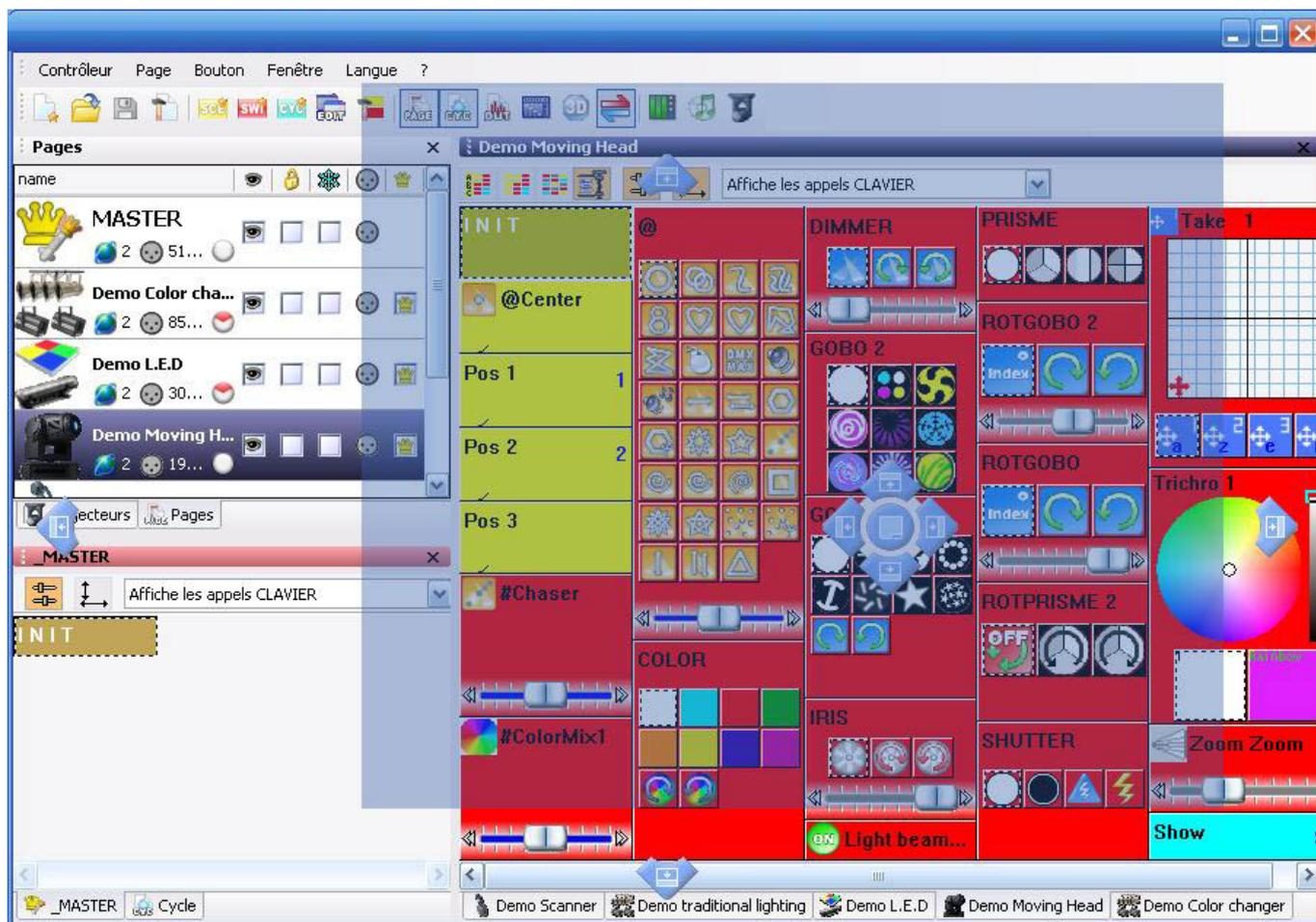
To software helps to find the correct position with the following tool. Moving the mouse on it enables to create a new tab or split the screen vertically or horizontally. The icon in the centre creates the tab and the other 4 icons split the window.
