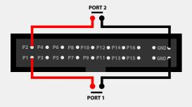
To activate a port, a brief contact of at least 1/25 second must be established between the ports (1...16) and the ground (GND) using the external HE20 connector.
