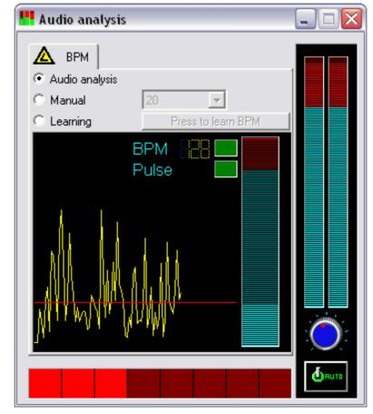
Right click on a scene button to switch it into BPM mode. When using an external sound-source, it is recommended to always check your PC recording track. In your Windows-mixer, the microphone track must absolutely be de-activated when an RCA connection to your computer sound-console is made. To boost your computer, Audio analysis should be run as a background task.
