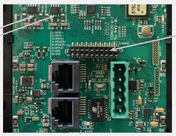
\* VIN pin 20 is not protected and should not be used
