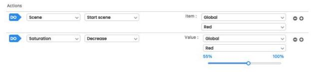
In summary our T-C-A trigger occurs at 12.00 everyday IF port 1 is pressed. When it's 12.00 and port 1 is pressed the Red scene in our Global zone activates at 55% saturation. You can see the complete trigger in the image below.
