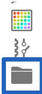
ESA Pro 2.1 paired with a DINA DR1 allows you to directly control the inbuilt relays. Relays in ESA Pro 2.1 are treated as single channel DMX devices, and consequently take up a channel in your DMX universe. You can import relays by clicking the switch icon. For more information, please consult the full ESA Pro 2.1 manual.
