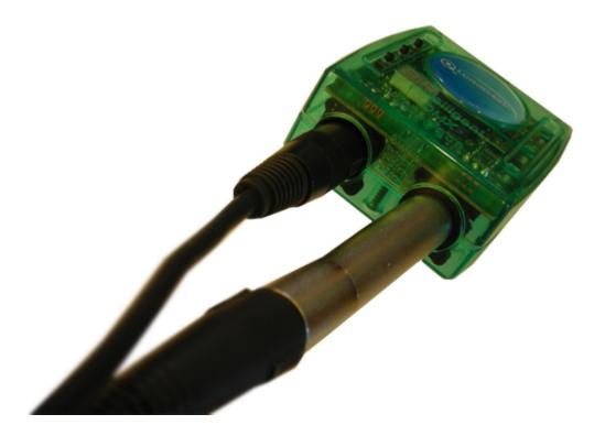
Now the interface is configured to have one DMX Output and one DMX Input. There is "PC" on the display and the red LED (showed by the arrow on the picture) is not blinking.
