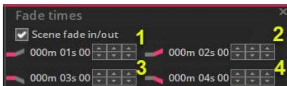
Whether to use the *fade in* or *fade out* is determined by the current DMX level of the fading channel. The *fade in* is used if the current value is lower than the value of the fading scene. The *fade out* is used if the current DMX value is higher than that of the fading scene.
