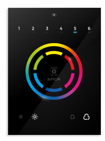
The STICK-CW4 programmable lighting controller, for RGB and RGBW lighting, has been designed around a touch sensitive color wheel. The controller is USB programmable from a PC or Mac using the ESA2 software.
