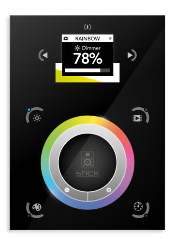
The feature rich STICK-DE3 has been designed to provide a control solution for the most demanding of projects and yet easy enough for anyone to use. The controller integrates a graphical color display, allowing scene photos to be displayed. Easily view the selected zone, scene name and design without the need to navigate through complex menus.
