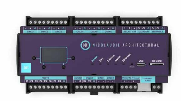
The DINA-DR1 is the latest lighting control solution from Nicolaudie Architectural. Our talented R&D team has worked a lot to design this all-in-one controller featuring multiple output protocols (DMX, Art-Net or SACN, LED Pixel, DALI), triggering and integration facilities, programmable memory for dynamic lighting sequences, remote control...
