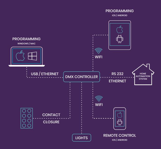
Most of the applications will use USB and DMX512 connections only, but the most demanding of our customers will also be able to interface additional devices through various connections: contact closures, UDP/TCP, RS232...
