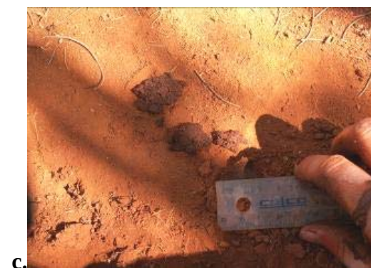
Figure 2.6 Determining soil texture: a. Making a caste from soil sample, b. Making a ribbon from soil sample, c. Measuring the ribbon from soil sample.
