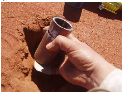
Figure 2.7 Collecting soil sample for bulk density assessment: a. hammering steel pipe into soil, b. removing soil from around the pipe, c. removing the soil sample.
