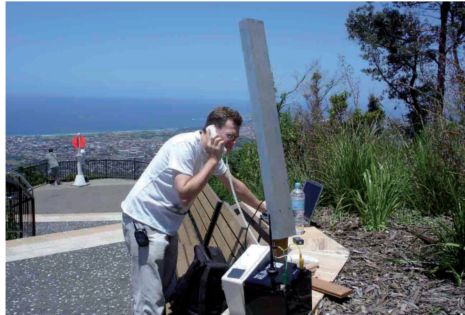
Figure 8.4.3.2: Long-range point-to-point setup with a waveguide antenna
