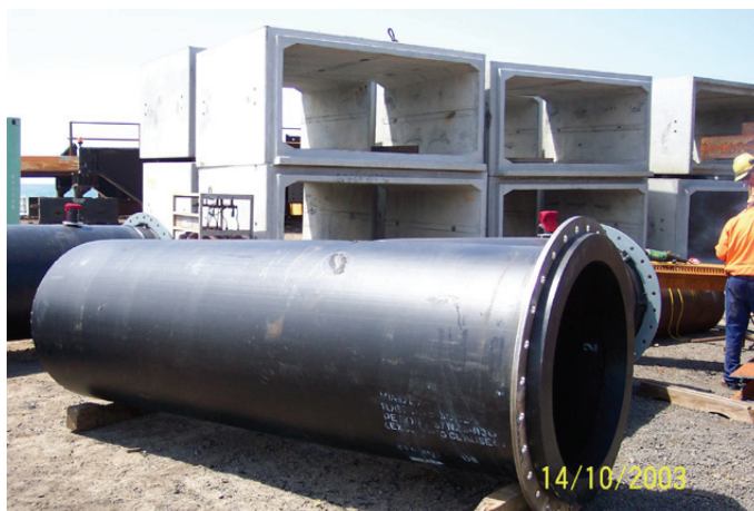
Figure 5: Stub flange and backing plate
