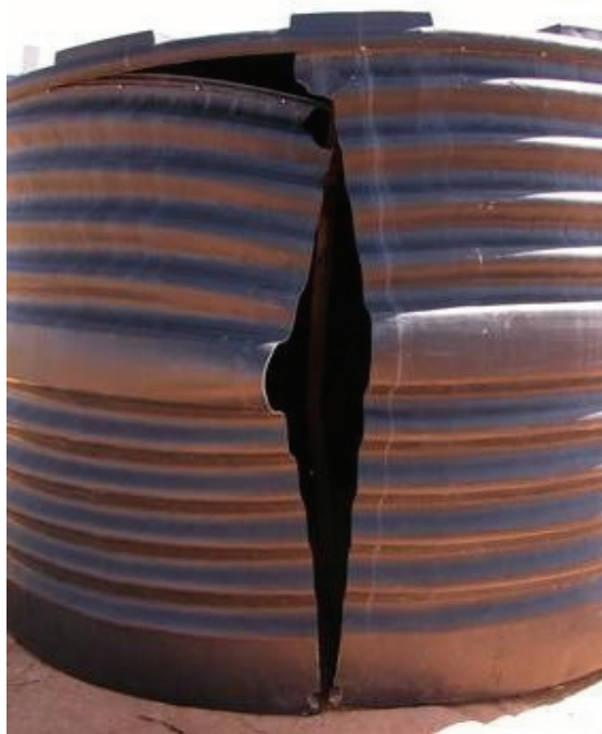
Figure 16: Splitting of poly tank with a vertical seam
