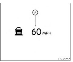
When passing another vehicle, the set speed indicator (A) will flash when the vehicle speed exceeds the set speed. The vehicle detect indicator will turn off when the area ahead of the vehicle is open. When the pedal is released, the vehicle will return to the previously set speed.
