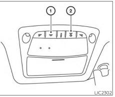
When the ON switch ① is pressed, the footwell lights (if so equipped), step lights (if so equipped), map lights and rear personal lights will automatically turn on and stay on for a period of time when:
