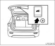
While holding the liftgate in position, push and hold the liftgate switch located on the liftgate for approximately 5 seconds or until two beeps are heard.
