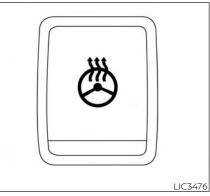
The heated steering wheel system is designed to operate only when the surface temperature of the steering wheel is below 68°F (20°C).
