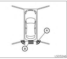
When the corner of the vehicle moves closer to an object, the corner sonar indicator (A) appears. When the center of the vehicle moves close to an object, the center sonar indicator (B) appears.
