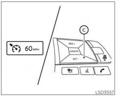
To set cruising speed, accelerate your vehicle to the desired speed, push the SET-  $\bigcirc$  switch and release it. (The color of the cruise indicator changes to green and set vehicle speed indicator comes on.) Take your foot off the accelerator pedal. Your vehicle will maintain the set speed.
