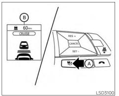
Operating vehicle-to-vehicle distance control mode
