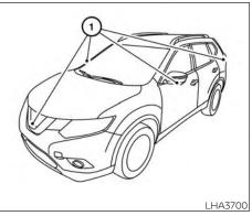
To display the multiple views, the Intelligent Around View Monitor system uses cameras located in the front grille, on the vehicle's outside mirrors and one just above the vehicle's license plate (1).
