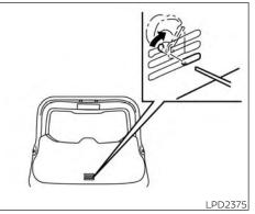
Manual liftgate release (if so equipped)
