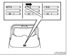
Power liftgate release (if so equipped)
