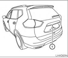
To display the rear view, the RearView Monitor system uses a camera located just above the vehicle's license plate ①.
