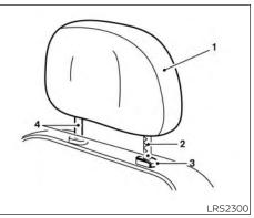
ADJUSTABLE HEAD RESTRAINT/ HEADREST COMPONENTS
