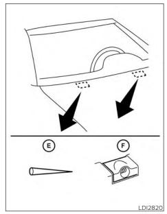
If you wax the surface of the hood, be careful not to let wax get into the washer nozzle  $(\mathbf{\hat{F}})$ . This may cause clogging or improper windshield-washer operation. If wax gets into the nozzle, remove it with a needle or small pin  $(\mathbf{\hat{E}})$ .
