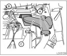
The viscous paper type filter element should not be cleaned and reused. Replace it according to the maintenance log shown in the "Maintenance and schedules" section of this manual.
