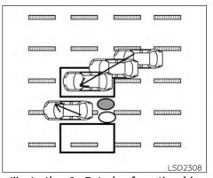
• The radar sensors may not detect a vehicle which is traveling at about the same speed as your vehicle when it enters the detection zone.
