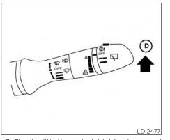
7. Finally, lift the windshield wiper and washer lever to the mist position () once and release. This action will cause the wipers to resume the set position.
