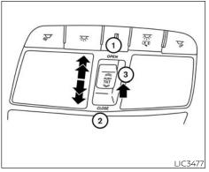
The moonroof will only operate when the ignition switch is placed in the ON position. The moonroof is operational for a period of time, even if the ignition switch is placed in the OFF position. If the driver's door or the front passenger's door is opened during this period of time, the power to the moonroof is canceled.
