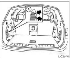
1. The jack and tool kit are located in the storage compartment to the left.
