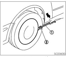
Removing wheel cover (if so equipped)
