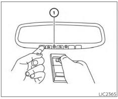
Position the end of your hand-held transmitter 1–3 in (2–8 cm) away from the HomeLink® surface, keeping the HomeLink® indicator light ① in view.
