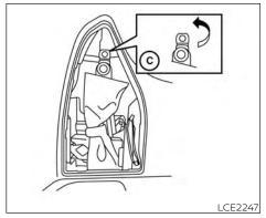
5. Remove the jack by turning the spindle (C) counterclockwise, relieving the pressure on the jack.
