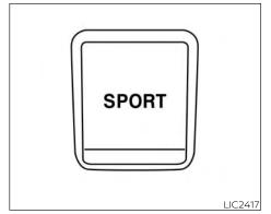
The SPORT mode switch adjusts the engine and transmission points to enhance performance. Push the SPORT mode switch on the instrument panel to activate. The SPORT mode indicator appears in the vehicle information display.
