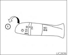
Autolight system (if so equipped) The autolight system allows the headlights to turn on and off automatically. The autolight system can:
