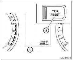
Odometer/Twin trip odometer
