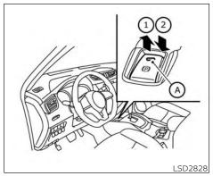
SWITCH TYPE (models with electronic parking brake system)
