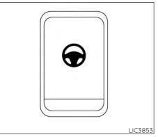
The Steering Assist switch is used to turn on and off the Steering Assist system that is activated using the settings menu of the vehicle information display.
