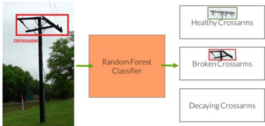
Training a neural network to identify asset locations in images and then a Random Forest classifier to sort overhead assets into health categories
