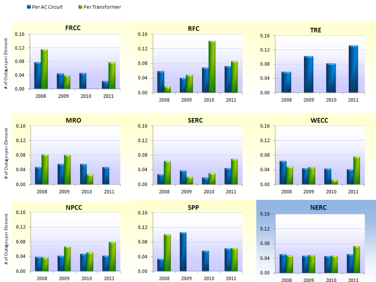
Figure 50: ALR6-13 Automatic Outages Initiated by Failed AC Substation Equipment by Regional Entity (Includes NERC-Wide)
