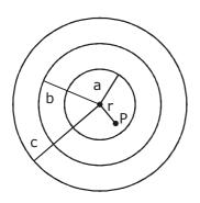
Potential at point P, V =  $\frac{kQ_a}{a} + \frac{kQ_b}{a} + \frac{kQ_b}{a}$  $\begin{array}{l} \because \ Q_a:Q_b:Q_c::a^2:b^2:c^2\\ [since \ \sigma_a=\ \sigma_b=\ \sigma_c] \end{array}$  $\therefore Q_{a} = \left[\frac{a^{2}}{a^{2} + b^{2} + c^{2}}\right] Q$  $Q_{b} = \left[\frac{b^{2}}{a^{2} + b^{2} + c^{2}}\right] Q$  $Q_{c} = \left[\frac{c^{2}}{a^{2} + b^{2} + c^{2}}\right] Q$  $V = \frac{Q}{4\pi \epsilon_0} \left[ \frac{(a+b+c)}{a^2+b^2+c^2} \right]$
