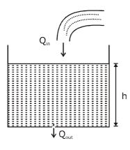
Since height of water column is constant therefore, water inflow rate (Q<sub>in</sub>) = water outflow rate
