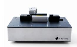
This modified version of the automatic AUTOCOATER 2™ is equipped with special clamps for recoating applications where only short lengths of fiber are available. A narrower positioning and shorter distance between the fiber clamps than in the standard version enables clamping and recoating of fibers as short as 124 mm without reducing the recoat length itself.
