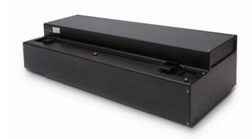
The AUTOSTRIPPER XL<sup>TM</sup> is designed for fast, chemical-free window stripping of optical fibers, using heated air to accomplish the demanding task of window stripping acrylate-coated fibers with diameters up to 550  $\mu$ m. The AUTOSTRIPPER XL<sup>TM</sup> is an extended version of the AUTOSTRIPPER 2<sup>TM</sup> and features longer strip lengths up to 500 mm.
