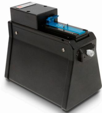
The CLEAVEMETER LIGHT™ is a non-contact interferometer designed for inspecting the end-faces of cleaved or polished optical fibers with cladding diameters of 125 µm to 800 µm. It gives immediate and precise information on important end-face properties such as flatness, perpendicularity, hackles and dust. Based on the NYFORS CLEAVEMETER 3D™ design, in addition to displaying sharp fringe patterns it also generates three-dimensional images of the cleaved fiber end.
