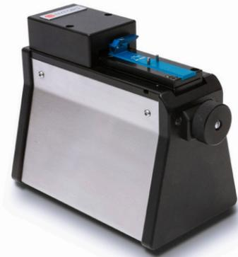
The CLEAVEMETER 2™ is a non-contact interferometer designed for inspecting the end-faces of cleaved or polished optical fibers with cladding diameters of 125µm to 1200µm. It gives immediate information on important end-face properties such as flatness, perpendicularity, hackles and dust. Sampling tests as well as continuous process documentation can be carried out both easily and quickly, making this an ideal instrument for cleaver inspection and optimisation.
