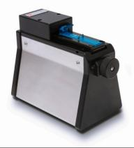
THE CLEAVEMETER 3D<sup>™</sup> is a non-contact interferometer designed for inspecting the end-faces of cleaved or polished optical fibers with cladding diameters of 125µm to 1200µm. It gives immediate and precise information on important endface properties such as flatness, perpendicularity, hackles and dust. Based on the NYFORS CLEAVEMETER 2<sup>™</sup> design, in addition to producing sharp fringe patterns it also generates three-dimensional images of the cleaved fiber end.
