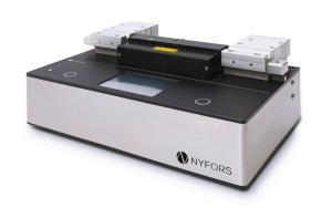
The RECOATER 2 XL™ is designed for recoating applications where the protective acrylate coating needs to be restored on long lengths of stripped fiber. It accommodates special silicone moulds that enable recoating of fiber sections up to 100 mm long.
