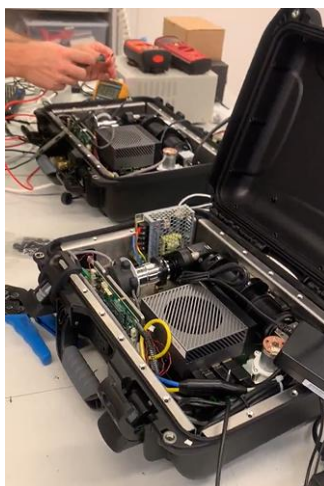
Figure 1. Microplastic sensors during its assembling at Leitat laboratory.
