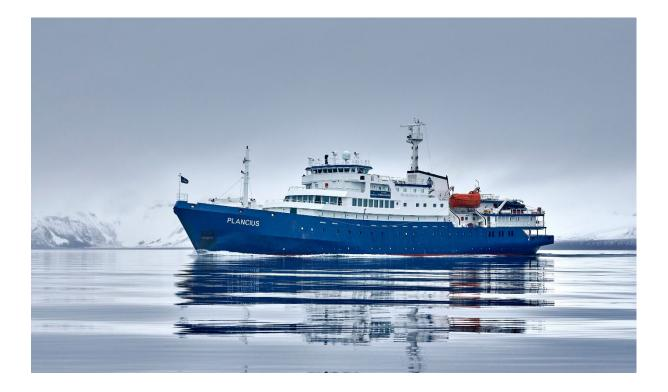
M/v *Plancius* was built in 1976 as an oceanographic research vessel for the Royal Dutch Navy and was named "Hr. Ms. *Tydeman*". The vessel was completely rebuilt as a passenger vessel in 2009 and complies with the latest SOLAS-regulations (Safety Of Life At Sea). M/v *Plancius* is 89 m long, 14.5 m wide and has a maximum draft of 5 m, ice class 1D, 10,5 knots average cruising speed and has 3 Diesel- Electric engines.
