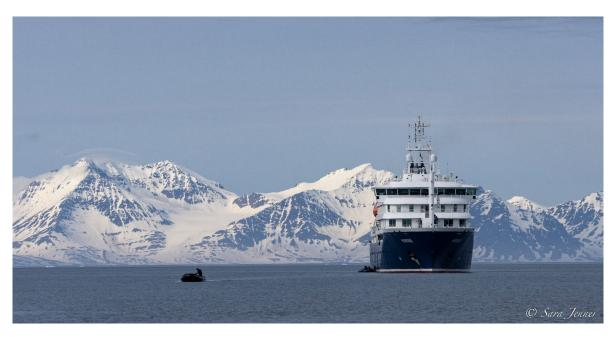
Hondius was built in 2019 in Brodosplit, Croatia. She is 107.60m long, 17,60m wide, and has a maximum draught of 5.3m. With a high ice class of PC6, a top speed of 15 knots, and three diesel generators, she sails on low sulfur marine gas oil (LSMGO) and has a capacity of 176 passengers in 83 cabins. This beautiful mid-century modern vessel carries 369m3 of fresh water and has a water plant producing 70m3 per day. Hondius is designed from the ground up for true polar adventure.
