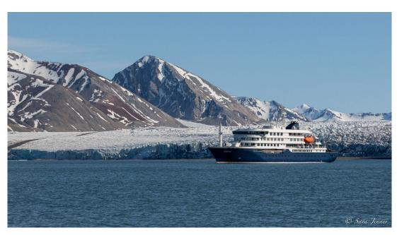
Hondius was built in 2019 in Split, Croatia. She is 107.6m long, 17.6m wide, and has a maximum draught of 5.3m. With an ice class of PC6, a top speed 15 knots, and three diesel generators, she sails on low sulfur marine gas oil and has a capacity of 176 passengers in 83 cabins. This beautiful mid-century modern vessel is designed from the ground up for polar adventure.
