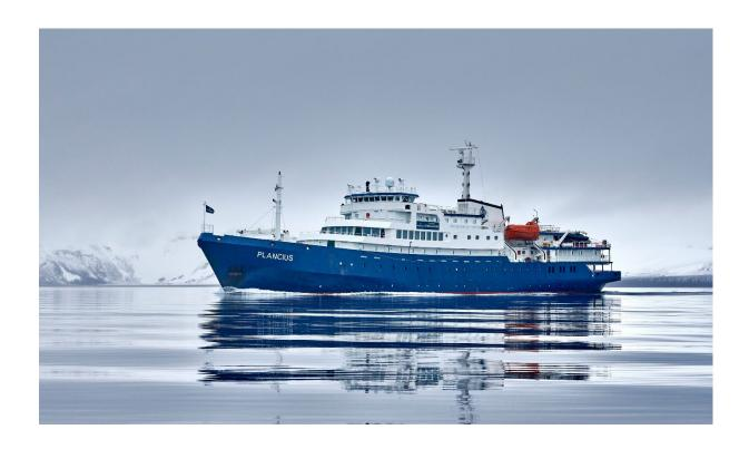
Plancius was built in 1976 as an oceanographic research vessel for the Royal Dutch Navy and was then named Hr. Ms. Tydeman. The vessel was rebuilt as a passenger vessel in 2009 and complies with the latest SOLAS-regulations (Safety Of Life At Sea). She is 89m long, 14.5m wide, and has a maximum draft of 5m. Her ice class is 1D, average cruising speed 10,5 knots, and she has three diesel-electric engines.
