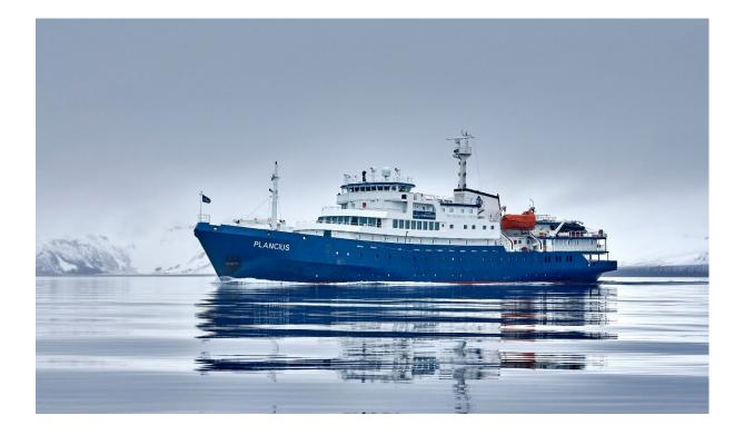
Plancius was built in 1976 as an oceanographic research vessel for the Royal Dutch Navy and was originally named "Hr. Ms. Tydeman." The vessel was rebuilt as a passenger vessel in 2009 and complies with the latest SOLAS (Safety Of Life At Sea) regulations. She is 89m long, 14.5m wide, and has a maximum draft of 5m. Her ice class is 1D and she averages a cruising speed of 10,5 knots using three diesel-electric engines.
