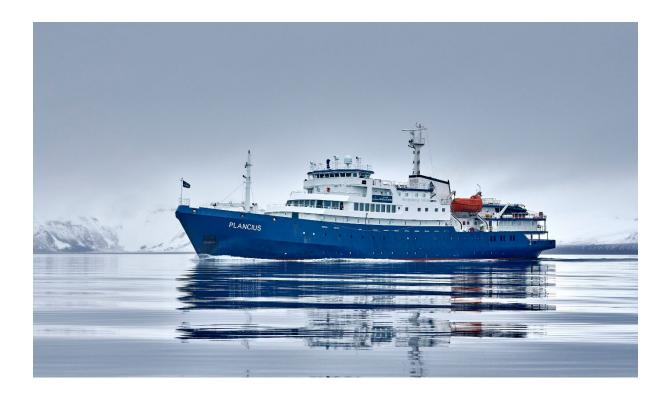
Plancius was built in 1976 as an oceanographic research vessel for the Royal Dutch Navy and was originally named Hr. Ms. Tydeman. The vessel was rebuilt as a passenger vessel in 2009 and complies with the latest SOLAS regulations. She is 89m long, 14.5m wide, and has a maximum draft of 5m. Her ice class is 1D and she averages a cruising speed of 10.5 knots using three diesel-electric engines.
