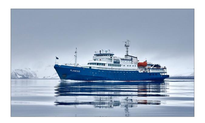
M/v Plancius was built in 1976 as an oceanographic research vessel for the Royal Dutch Navy and was named "Hr. Ms. Tydeman". The vessel was completely rebuilt as a passenger vessel in 2009 and complies with the latest SOLAS (Safety Of Life At Sea) regulations. She is 89m long, 14.5m wide, and has a maximum draft of 5m. Her average cruising speed is 10,5 knots on three diesel-electric engines.
