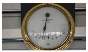
To breathe some fresh air, a walk up to the bridge was a must. There the clinometer was measuring the rolling of the ship; readings oscillated from 10° to 16° on average with peak of 20°-22°. Quite a dance for most of us who had to hold firmly on the rails inside the ship.
