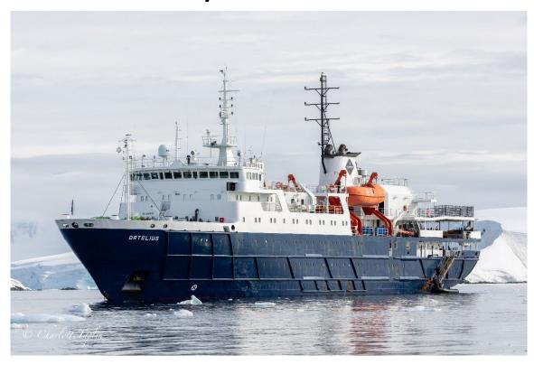
M/v Ortelius was built in 1989 it served as a special-purpose vessel for the Russian Academy of Science named "Marina Svetaeva". The vessel was completely rebuilt as a passenger vessel in 2019 and complies with the latest SOLAS-regulations (Safety of Life At Sea). M/v Ortelius is 90,95 m long, 17.2 m wide and has a maximum draft of 5,4 m, ice class UL1 (Equivalent to 1A), 10,5 knots average cruising speed and propulsion is 6 ZL 40/48 SULZER.
