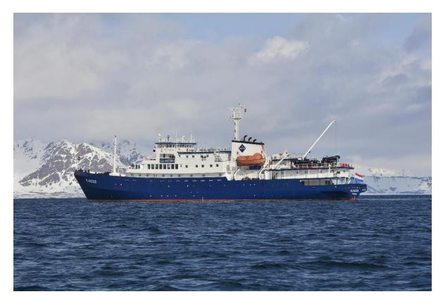
M/V *Plancius* was built in 1976 as an oceanographic research vessel for the Royal Dutch Navy and was named "Hr. Ms. *Tydeman*". The vessel was completely rebuilt as a passenger vessel in 2009 and complies with the latest SOLAS-regulations (Safety Of Life At Sea). M/v *Plancius* is 89 m long, 14.5 m wide and has a maximum draft of 5 m, ice class 1D, 10,5 knots average cruising speed and has 3 Diesel- Electric engines.
