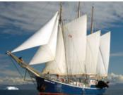
MV PLANCIUS Registered: The Netherlands Length: 89 meters Breadth: 14.5 meters Draft: 5 meters Ice class: 1D Displacement: 3,211 tons Propulsion: 3x Diesel-Electric Average cruising speed: 10,5 knots Passengers: 108 in 50 cabins Crew, guides, doctor: 37 / 8 / 1 Various decks refurbished 2009-2018-2019
