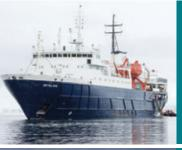
MV HONDIUS Registered: The Netherlands Length: 107.6 meters Breadth: 17.6 meters Draft: 5.30 meters Ice class: PC 6 (equivalent 1A-Super) Displacement: 5,590 tonnes Propulsion: 2 x ABC main engines; total 4,200 kW Design operation speed: 15 knots Passengers: 170 in 80 cabins Staff & crew: 72 New build 2019
