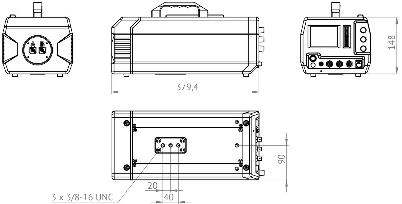
**Dimension of the autofocus Fiber Head without objective lens:**
