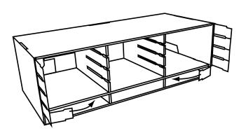
8. Fold the bottom SIDEWALLS of the BASE inward. Insert the other SHELVES the same way, folding inward the SIDEWALLS as before.
