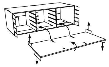
7. Fold inward the SHELF then back-fold the small side flaps. Insert a SHELF into the bottom slots of the DIVIDER.
