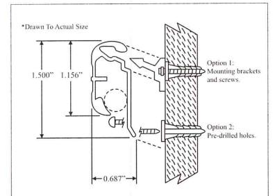
Grip-a-Strip offers a unique mounting bracket system. The extension has a channel groove located on the back that snaps into the plastic mounting piece. This bracket provides significant stability and is mounted out of sight when installed. In lieu of the mounting bracket system, holes can be pre-drilled in the flange for use with either standard or theft-proof screws.
