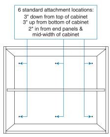
Locate first Wall cabinet, aligning outermost edge with outermost edge of Base cabinet directly below.
