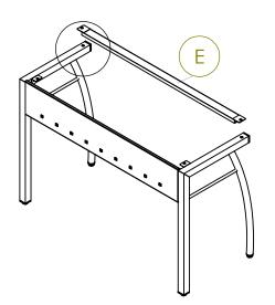
ATTACH SUPPORT BAR - DO NOT TIGHTEN
