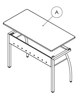
PLACE TOP PANEL ON LEG ASSEMBLY DO NOT TIGHTEN
