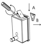
Unscrew the set screw inside the back of dispenser, and take out the wall bracket
