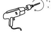
3. Drill the holes for plastic fixing
