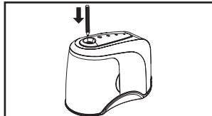
2. Insert a pencil into the slot on the top to get the pencils sharpened.
