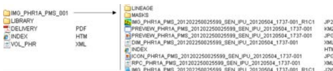
Figure 4.5: Example of DIMAP V2 Structure
