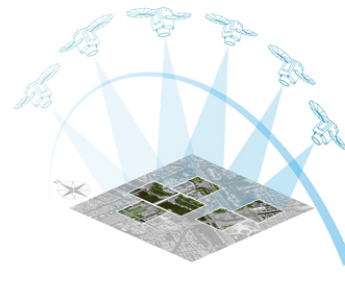
Multiple acquisitions Multiple acquisitions over a given area, typically ten images over an area of 100 x 200 km
