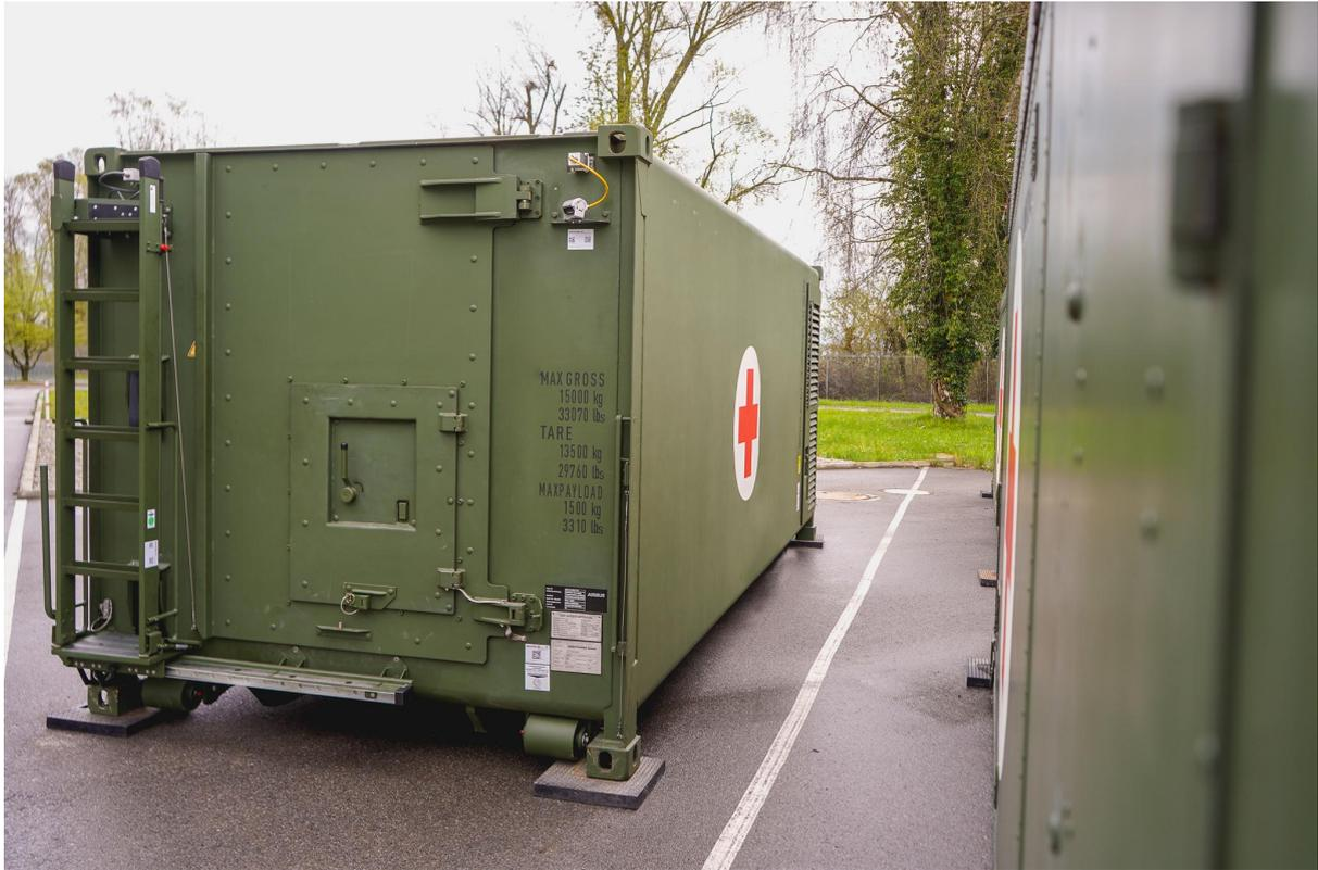
*The protected-wounded transport container is based on the international ISO standard 20-foot container.*
