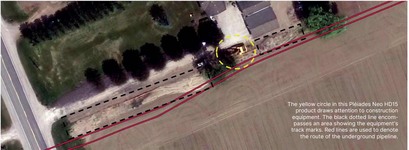
The yellow circle in this Pléiades Neo HD15 product draws attention to construction equipment. The black dotted line encompasses an area showing the equipment's track marks. Red lines are used to denote the route of the underground pipeline.
