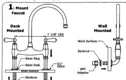
Ensure the mixer is orientated correctly, levers should rotate to point forward. After removing backnuts, place complete faucet through 01" holes at 7. 7/8" centers (do not remove unions from body) - product is fitted with straight unions, distance must be exact. Secure mixer with a suitable faucet wrench.
