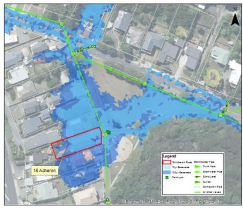
ISSUE: Debris blockage and low network capacity (multiple pipes with less than annual rainfall event capacity) leading to frequent property flooding (up to 8 properties) and a habitable floor flooding event at least every 3-6 years.
